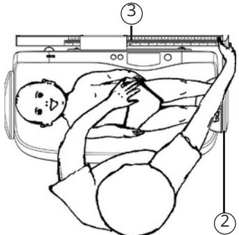
2. Use your right hand to move the foot support (2) towards the baby's feet. Rest the baby's feet on the foot support while doing so. With your left hand keep the baby still on the weighing tray.
