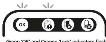
Green 'OK' and Orange 'Leak' indicators flash
