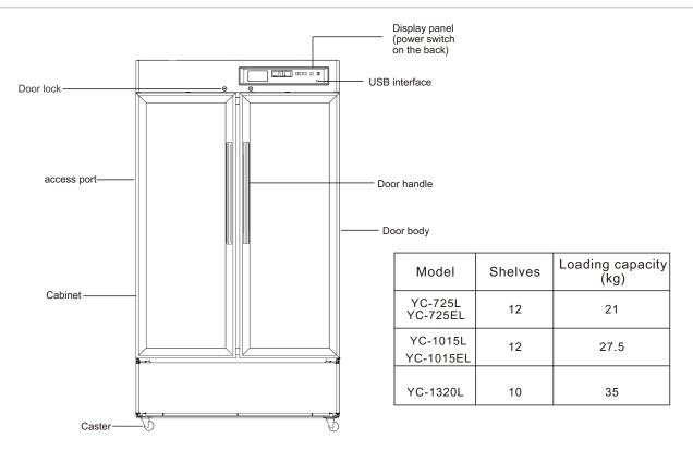
Figure V YC-725L((It can be used as reference for YC-725EL, YC-1015L, YC-1015EL, YC-1320L)
