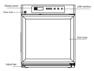
Figure I YC-55L (It can be used as reference for YC-55EL, YC-56L, YC-56EL, YC-75L, YC-76EL)
