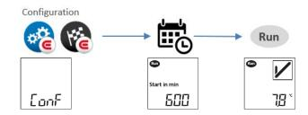
**CAUTION!** When re-starting or re-configuring from stop mode, **ALL RECORDED DATA** in the logger will be **DELETED**!
