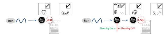
You can apply the two stop options mentioned above in parallel during the configuration (the logger can be stopped by one or the other method).
