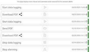
For "Download PDF" entries, the PDF reports can be called up by tapping on the "Share" symbol and displayed using an installed PDF reader.
