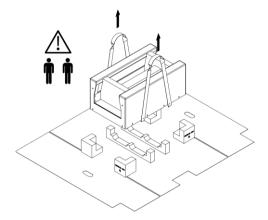
Remove the Allen key from the lifting strap.
