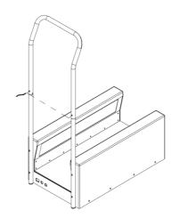
Place the steps next to the scanner, align the mounting holes with the holes at the sides of the scanner, and secure them using the four knobs. Adjust the steps until they are supported by the floor, fasten the knobs.
