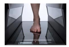
Each of the four lasers projects a line onto the foot from several angles. The eight monochrome cameras capture the laser projections.
