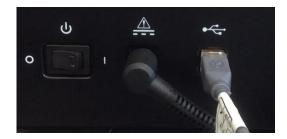
Connect the USB-A plug side of the cable (flat rectangular plug) to a free USB port on your PC.
