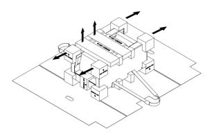
Lift the scanner with two persons using the attached straps.
