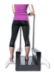
Roughly position the center of the foot in the center of the three white markers to obtain the best scan result.
