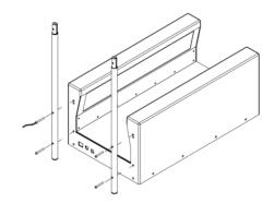
Slide the handle bar over the extension rods until the hex screws are visible through the holes in the handle bar.
