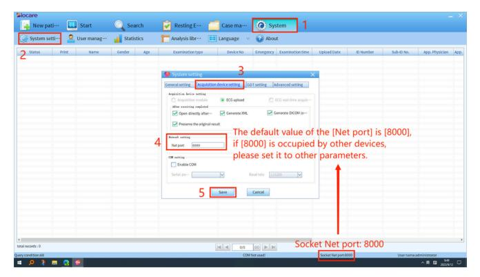
2. Please note that if you change the [*Net port*] parameter of ECG1000 on your computer, you will need to change the [*Port*] parameter in [*Menu*]-[*System setting*]-[*Server setting*] of the ECG machine.
