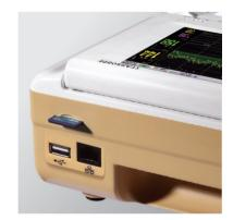
Support data storage and software upgrading by external USB disk. External SD card optional, for data transfering.
