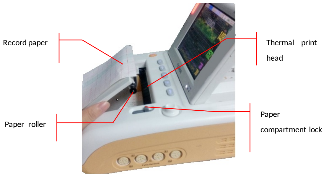
Fig 11-1 Loading record paper
