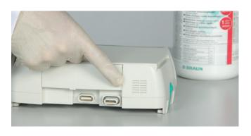
Make sure that no liquid is leaking into the ventilation or connectors. Let the device at least one minute to dry after cleaning / disinfection.
