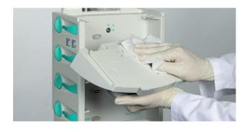
In case of heavy contamination remove cover – unlock the locking button and remove the SpaceCover. Remove visual contamination on the SpaceCover and the guide rail as described above. Dispose the cloth after usage.
