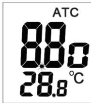
4. Press „“ to freeze current readings. The „“ icon will appear on the LCD and the small dot will not flash. Press „“ again to release the hold mode.
