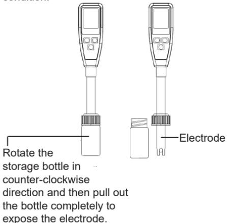
2. Dip the electrode into the test solution. Press „“ to power on the meter and tilt it to get a stable reading.
